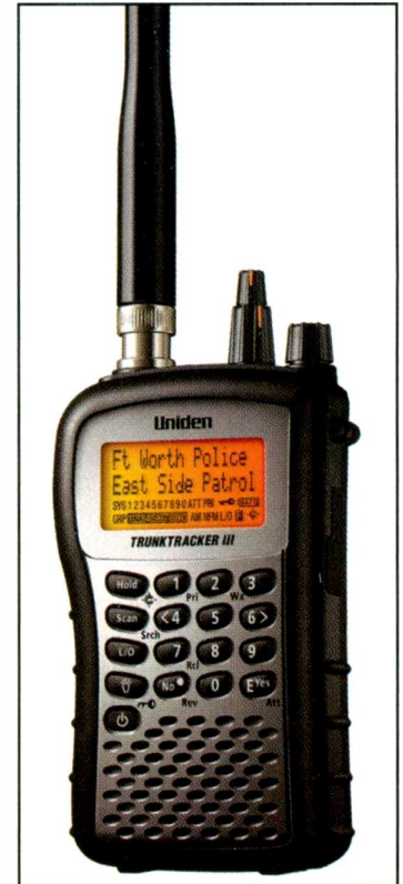
Capture it all with the new Uniden BC246T compact handheld scanner, but in your zeal to program any and all frequencies, don't forget the basics: 156.80 MHz and others are often a wealth of information.
