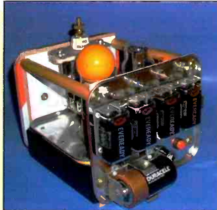
Photo G. Rear apron view shows the batteries mounted in metal Keystone brand battery holders. Four 9-volt batteries provide the B+ for the regenerative detector and audio stage. A single D cell is for the 1H4 battery triode tube 1-1/2 volt filament.
