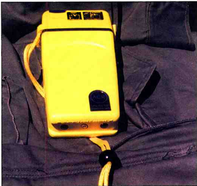
A PLB, such as this one, transmits on 121.5 MHz and data bursts on 406.028 MHz.
