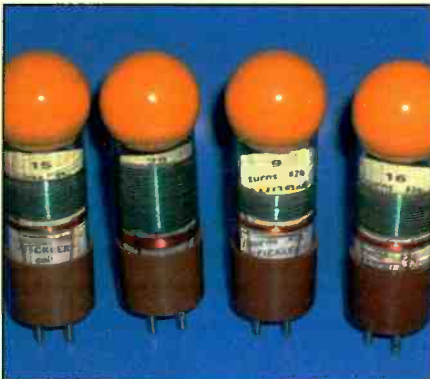
Photo H. Here's a set of finely crafted four-pin plug-in coils for the Boy's First Receiver. Reader Bob Ryan also made these coils.
